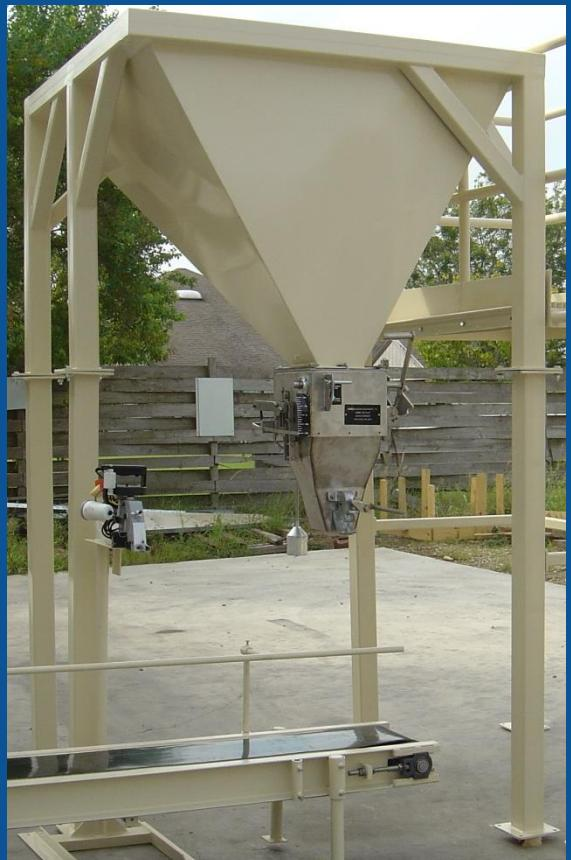
Self Standing Supply Bin with Interfacing Flange to Support the GB Bagging Scale.
